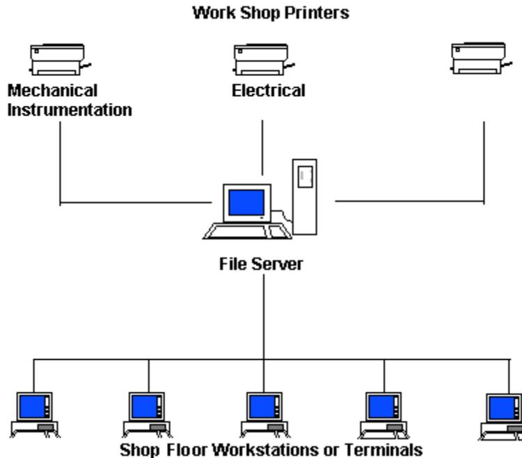
In this installation, the production operation requires support from three separate service groups, each of which operates from a dedicated workshop. There are a number of shop floor terminals located strategically, around the production area. A networked printer is installed in each workshop. The main software package is installed on the file server.
